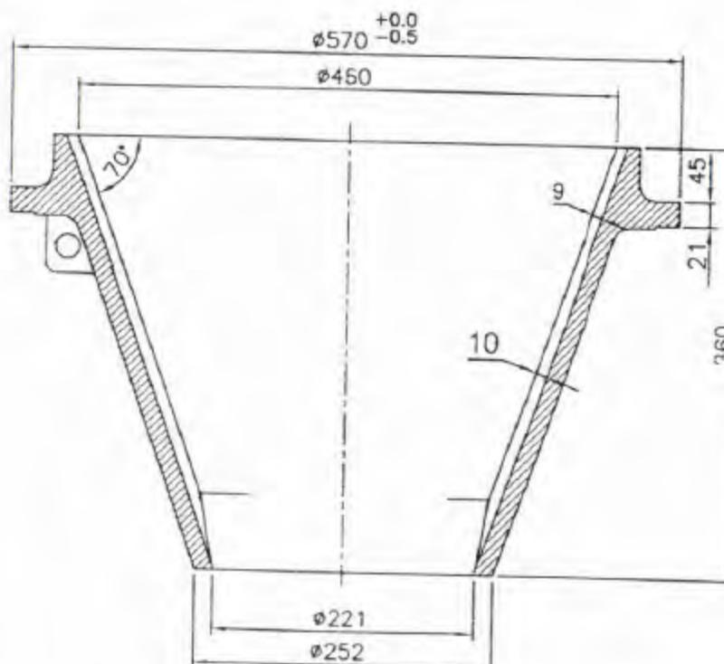
SECTION-A-AALL DIMENSIONS ARE IN MM**Rotor**
